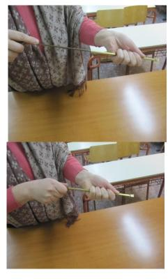
Sequential phases of the metal rod's movement into the metal tube. Please hold firmly with one hand the metal tube. With the other hand move the metal rod back and forth into the metal tube, for one minute.
